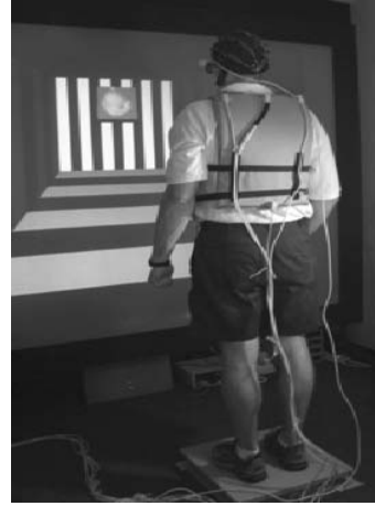
FIG. 1. Experimental set-up incorporating VT, force plate and Flock of Birds Motion tracking technologies.
